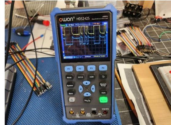
Figure 3: Owon Handheld scope shows the Can-H and Can-L signals.
