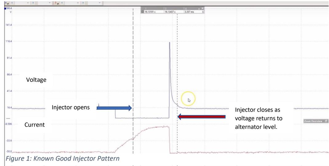
The trace also shows the overall time the injector is open. Fuel injectors respond to a magnetic field just as any coil does. Once the voltage signal is turned off, the current drops rapidly as the coil energy decays. However, the collapse of this magnetic field induces a high voltage spike of over 110 volts for a very short amount of time. Then the injector finally closes as this voltage decreases. You can see this by looking at the second small dip in the voltage noted by the red arrow.
