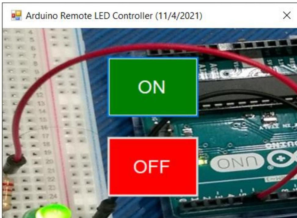
This is called "Blinky" and it uses a Windows form C# app to control an LED on a breadboard that is managed by an Arduino UNO.
