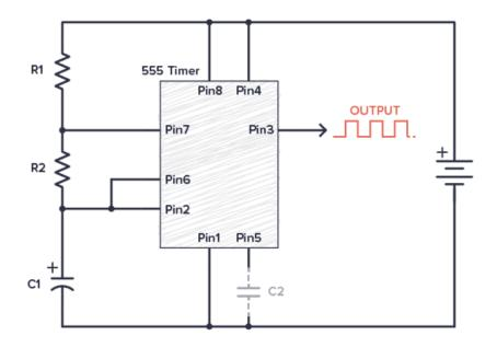
Oscillator mode to blink a light, create sound, generate a clock, and much more.
