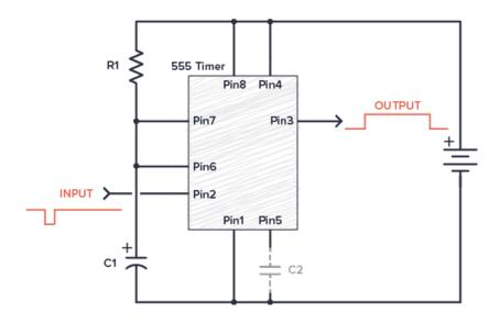
One-shot mode to create a pulse of a specific length. Can convert the negative edge of one tiny pulse, or a series of short pulses, into one pulse.
