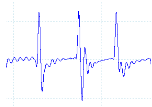
Figure 8: Knock Sensor Trace With 15Hz Low Pass Filter Installed
