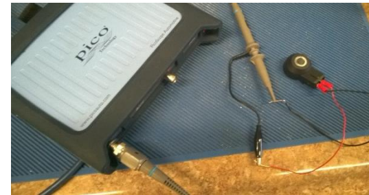
Figure 3: Bench Testing the Knock Sensor
